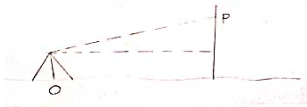
FIG. Measurement of vertical angle by theodolite
