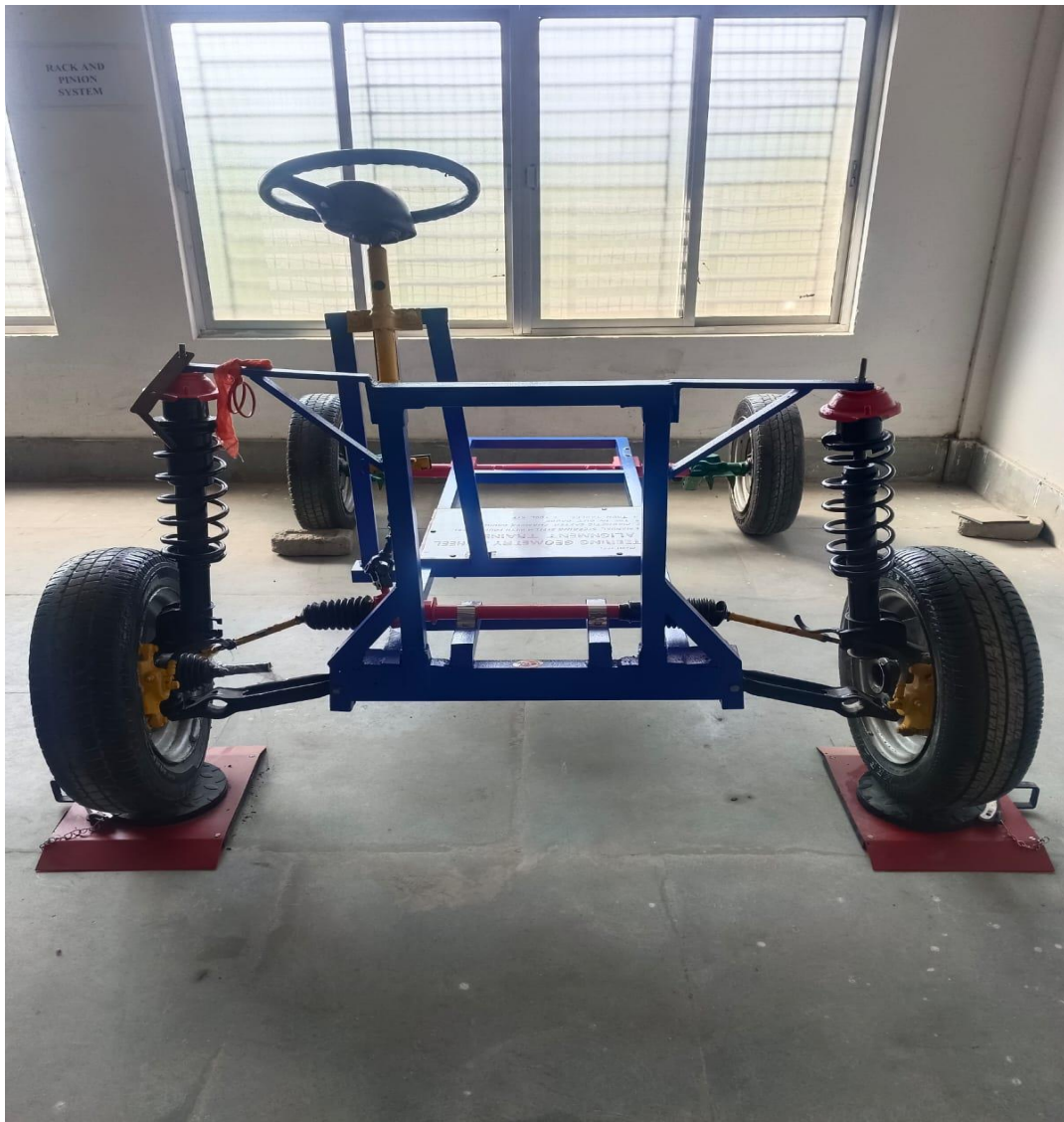
(A model of steering geometry is located in vehicle dynamics lab ) 19
