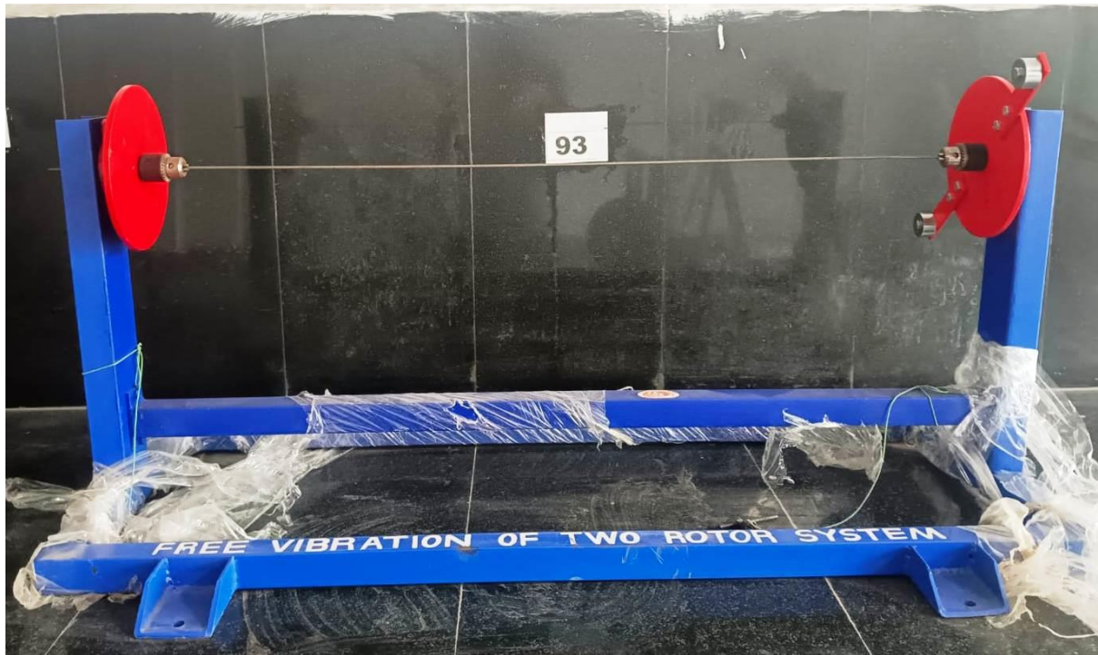
(Free vibration of two rotor system placed in vehicle dynamics lab)
