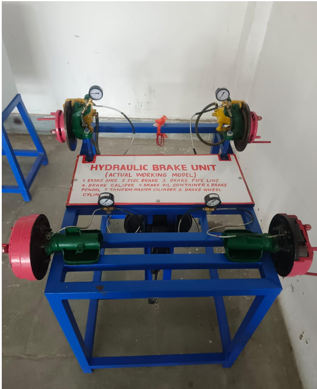
(A working model of hydraulic braking system located in dynamics lab)
