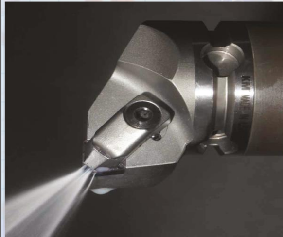
(a) A turning insert with coolant applied through the tool; (b) comparison of temperature distributions for conventional and through-the-tool application. Source: Courtesy of Kennametal, Inc.
