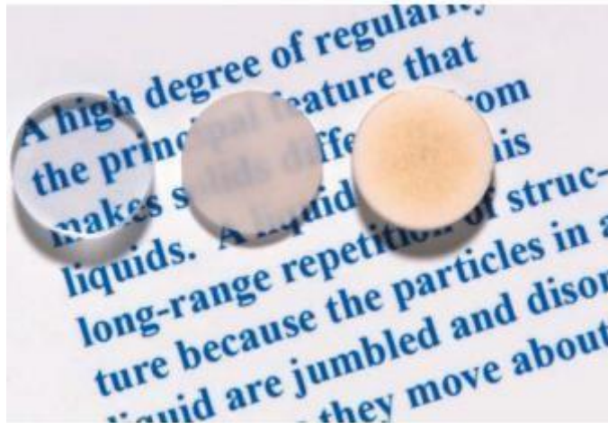
Figure 1. Three thin disk specimens of aluminum oxide that have been placed over a printed page in order to demonstrate their differences in light-transmittance characteristics. The disk on the left is transparent (i.e., virtually all light that is reflected from the page passes through it), whereas the one in the center is translucent (meaning that some of this reflected light is transmitted through the disk). The disk on the right is opaque—that is, none of the light passes through it. These differences in optical properties are a consequence of differences in structure of these materials, which have resulted from the way the materials were processed. (Specimen preparation, P. A. Lessing; photography by S. Tanner.)
