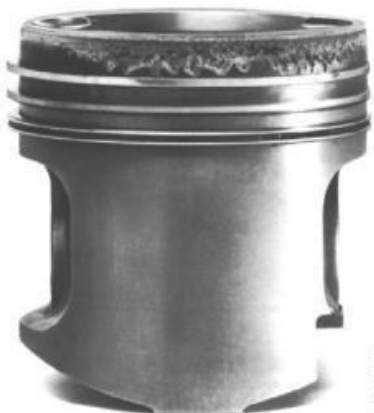
Piston Damage by knock
